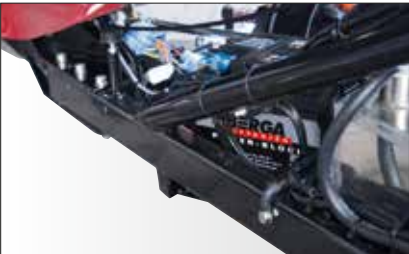
Frame: Plastic coated with car standards (salt spray test 600 h). Increased corrosion protection by 4-phases handling. Thick wall-thickness. Buckling resistant and optimal riding quality.
