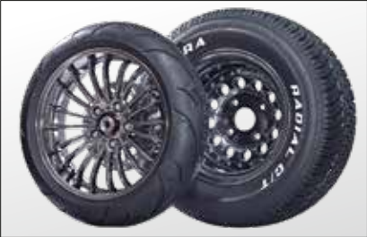
Wide-base tyres: Rear 295/50 with rim protection on 10x15 rims.
